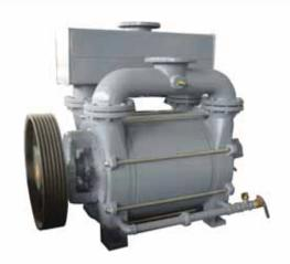
All of our liquid ring pumps handle wet or dry gases, with high tolerance to liquid carry over. The LR1A Series has an enhanced bearing design enabling reduced internal clearances for improved efficiency. Pumps are available in cast iron and 316 stainless steel construction as standard with other materials and corrosion-resistant coatings available. All are tested to DIN 28431:1987 and are available as part of ATEX Category 1 and 2 T4 systems.
